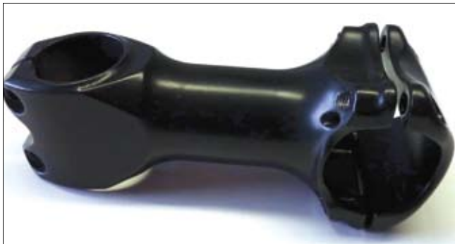
The solid magnesium bicycle stem extrusion is machined out of magnesium alloy AZ80, and then receives a pre-treatment and a ceramic paint layer prior to assembly. © Photo courtesy of Morgo Magnesium Ltd. Used with permission.
