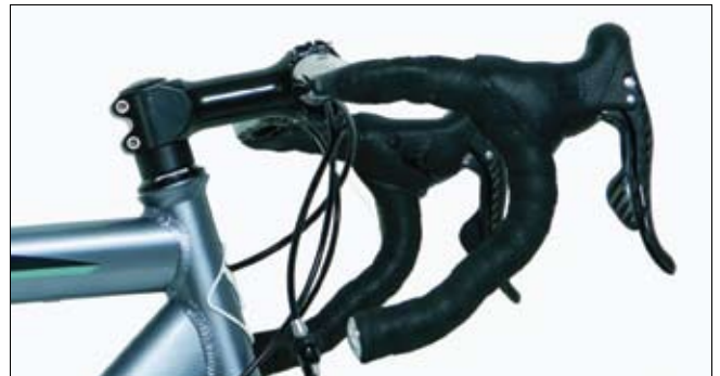
The magnesium stem extrusion, located between the fork and handlebars, is critical to absorbing vibrations at the front of the bike for a smoother ride and better control. © Photo courtesy of Morgo Magnesium Ltd. Used with permission.
